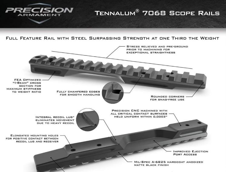
FULLY MACHINED FROM ULTRA HIGH STRENGTH TENNALUM<sup>®</sup> 7068 OFFERING THE STRENGTH OF STEEL AT ONE THIRD THE WEIGHT
