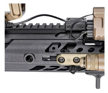
6. Place the left and right clamps over the U-bracket and use the included screws to secure them. Alternate tightening the clamps in place. Once finger tight, torque to 15 inch lbs.
