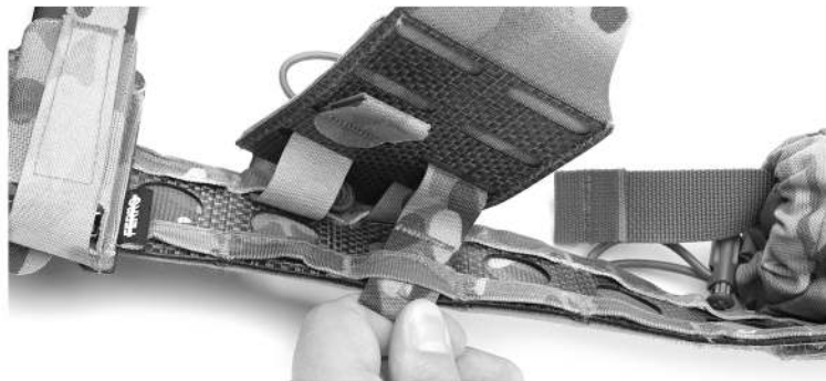
3. WEAVE THE PULL TAB THROUGH THE NEXT ROW OF MOLLE WEBBING
