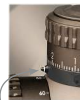
Turret in second turn of rotation (partially extended).
