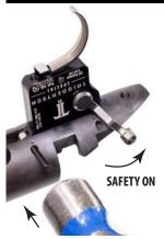
4a) Insert the trigger assembly and gently tap the front trigger pin in, from right to left. Ensure that the pin is not contacting the bolt release as this can jam the bolt catch, which is dangerous.
