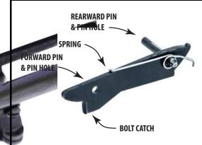
If your bolt catch assembly has come apart, assemble the bolt catch, spring, and pin, prior to re-installing it in your firearm. Slide the assembly into the slot as shown in Step 2 and gently tap the rearward pin in, to hold the bolt catch assembly in place.
