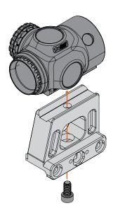
Insert each Clamp Screw through a Washer. Then insert them through the FAST™ MicroPrism mount and thread them into the Rail Clamp. Secure screws using a T25 bit driver. Lightly snug all screws before applying final torque to any. Torque to 35 in-lbs (4 Nm).
